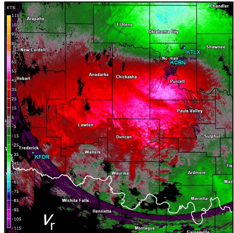
**Widespread** light precipitation covered most of the state on **December 13<sup>th</sup>, 2018**. The HSE are most effective on this type of weather (low-to-medium SNR).
